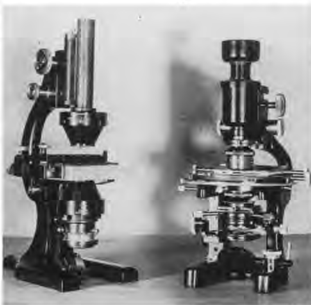
FIG. 2. Apochromatic reflecting-type microscope lenses in conventional stands: 0.4 NA objective lens (left); 0.72 NA objective lens (right); identical lenses used as condensers.
